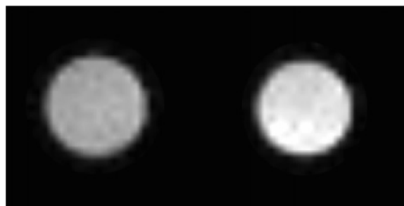
Figure 8. Internalized quantum dots produce MRI contrast. T_1 -weighted images from tubes containing cell lysates show that lysates of cells that have been incubated with quantum dots (right) show significant contrast enhancement as compared to cells that have not been exposed to quantum dots. These samples were from cells in the same experiment shown for the optical uptake studies of Figures 6 and 7. Images are 0.5 cm in diameter.
